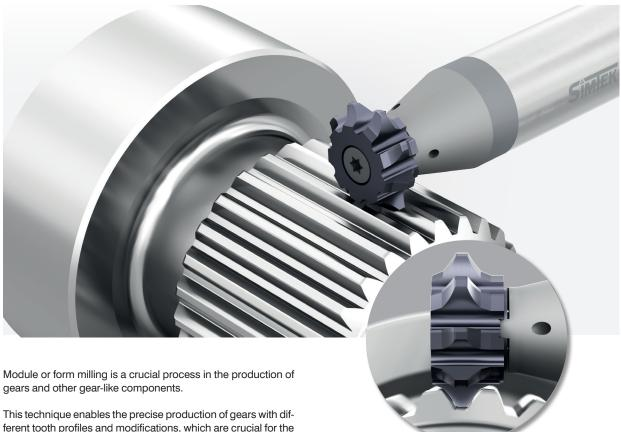
ferent tooth profiles and modifications, which are crucial for the performance and functionality of machines and transmissions.
